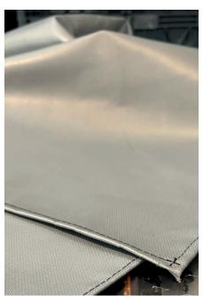
Wellplast® FIRE PROTECT is made from silicon and glassfiber.
